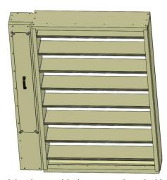
The walls of the casing which carried the damper blades are equipped with a 240 mm wide self-adhesive layer. The two other remaining walls contain a 15 mm deep V-groove which acted as damper blade stops.
